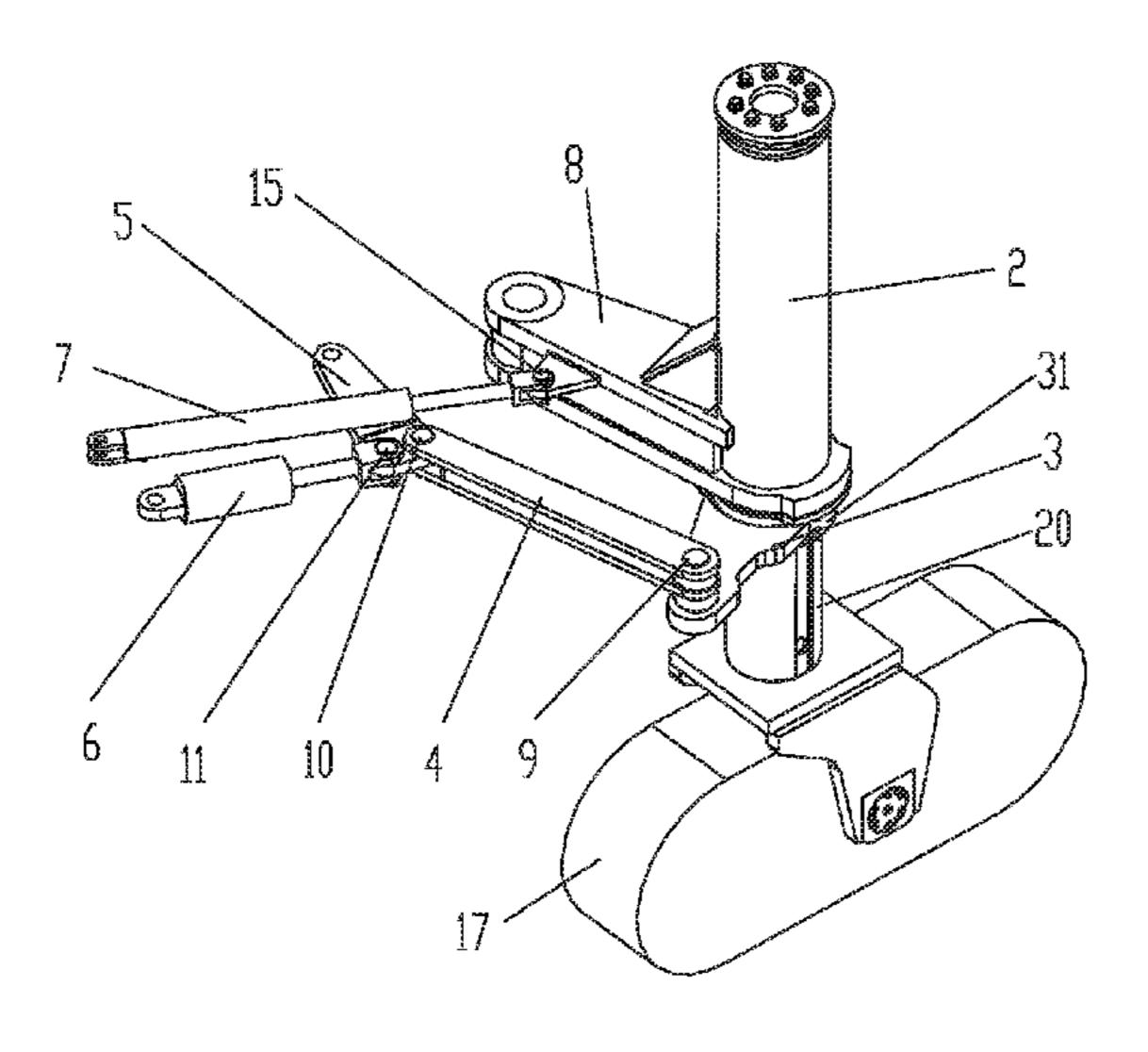
the first guiding rod is hinged to one end of the steering rod, and the other end of the steering rod is connected to the support leg interior sleeve.
