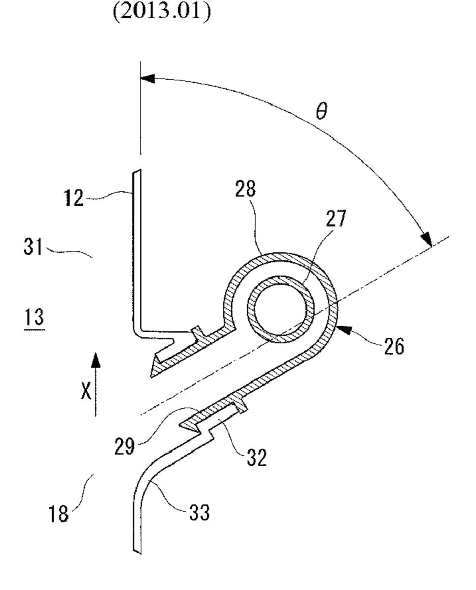
and a primary-air introducing unit of the aspirator is installed by being diagonally inserted into the boss portion.
