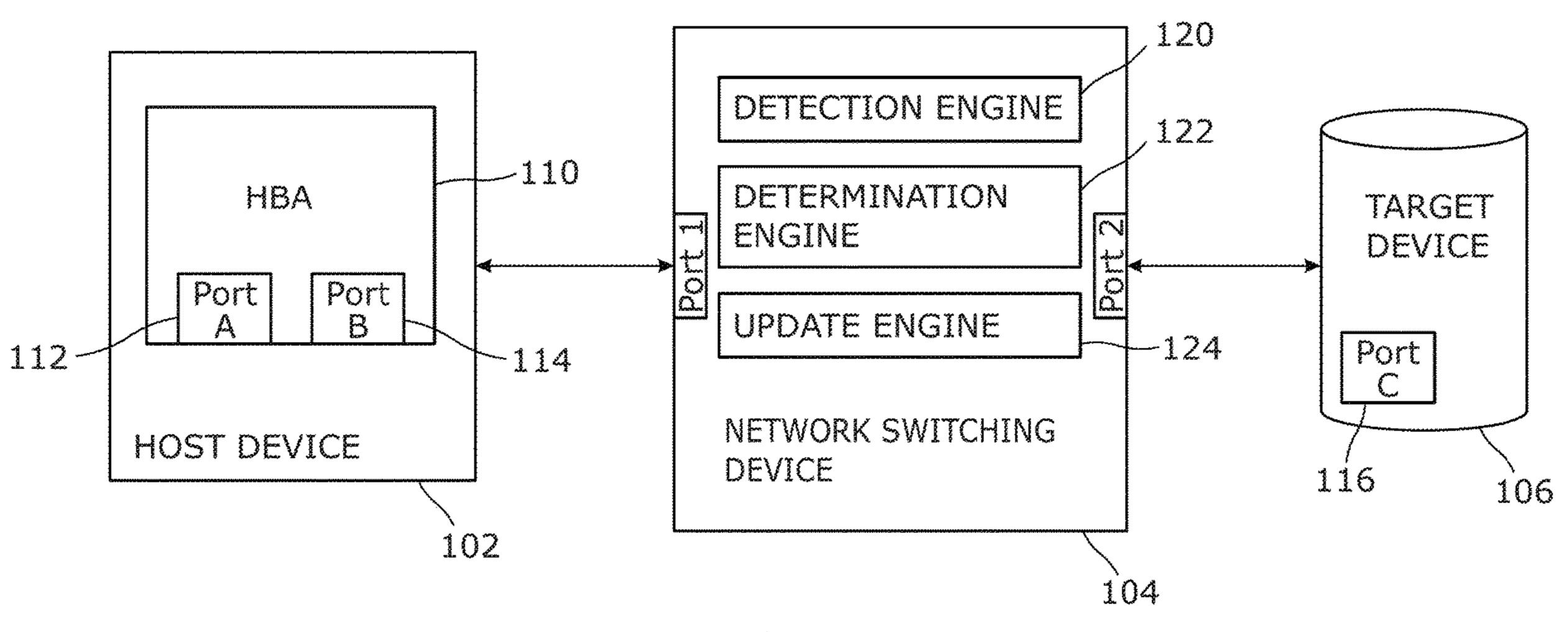
replace the ID of the prior HBA port with an ID of the new HBA port, for the zone that the prior HBA port belonged to.
