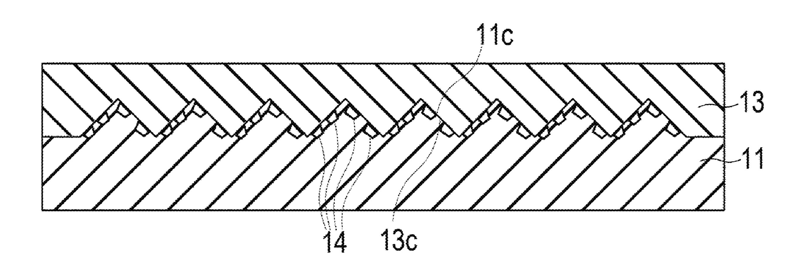
concavoconvex shape being formed on a surface of the positive electrode current collector that is in contact with the positive electrode active material layer. In the concavoconvex shape in the positive electrode current collector, at least a part of the positive electrode conductive member 14 that is in electrical contact with the conductive filler exists in the positive electrode current collector beyond the surface of the positive electrode current collector.
