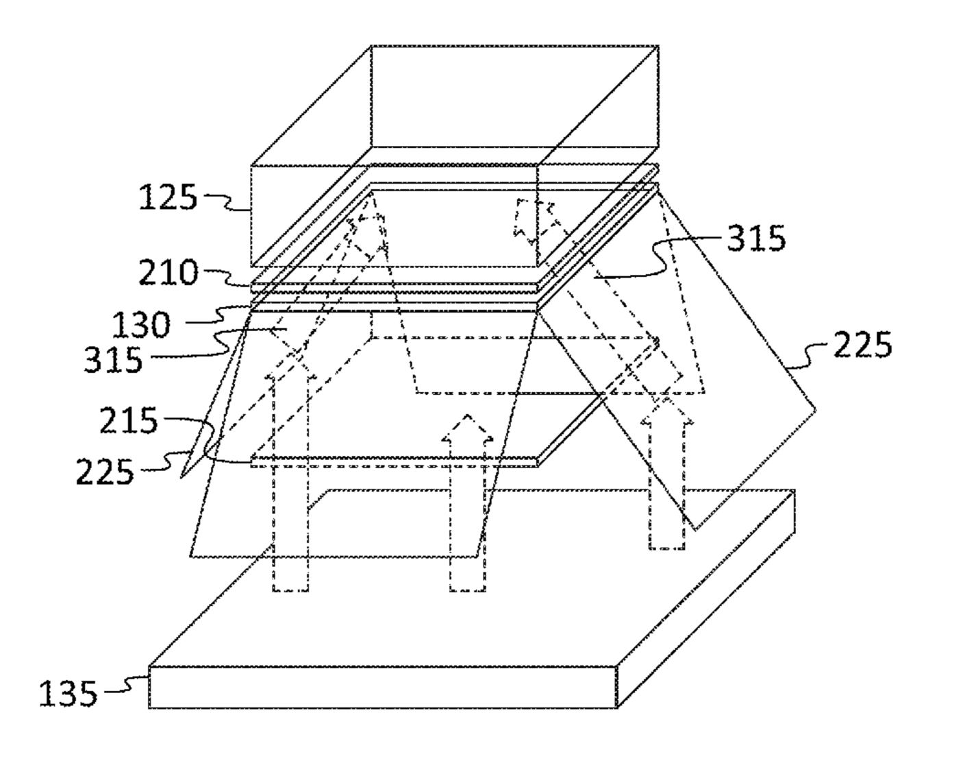
to reflect the light from the light source around the blocker and through the mask and into the reservoir. The blocker is positioned to block a straight path of light from the light source to the mask.
