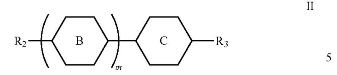
In the compound represented by formula II, R<sub>2</sub> and R<sub>3</sub> each independently represent an alkyl group having a carbon atom number of 1-10, an alkenyl group having a carbon 10 atom number of 2-10, an alkoxy group having a carbon atom number of 1-10, and any one or more non-connected CH<sub>2</sub> in groups R<sub>2</sub> and R<sub>3</sub> may be substituted with cyclopentyl, cyclobutyl, cyclopropyl, or —O—;
