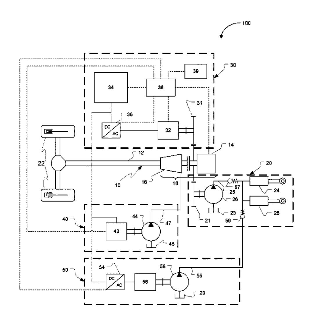
recharge the electric energy storage device, and that can subsequently stop the engine again when the electric energy storage device has reached a threshold 10 charge level. The electric energy storage device also powers at least one of: integral vehicle equipment; peripheral vehicle equipment; or an electrical outlet circuit with a socket for external plugin equipment.
