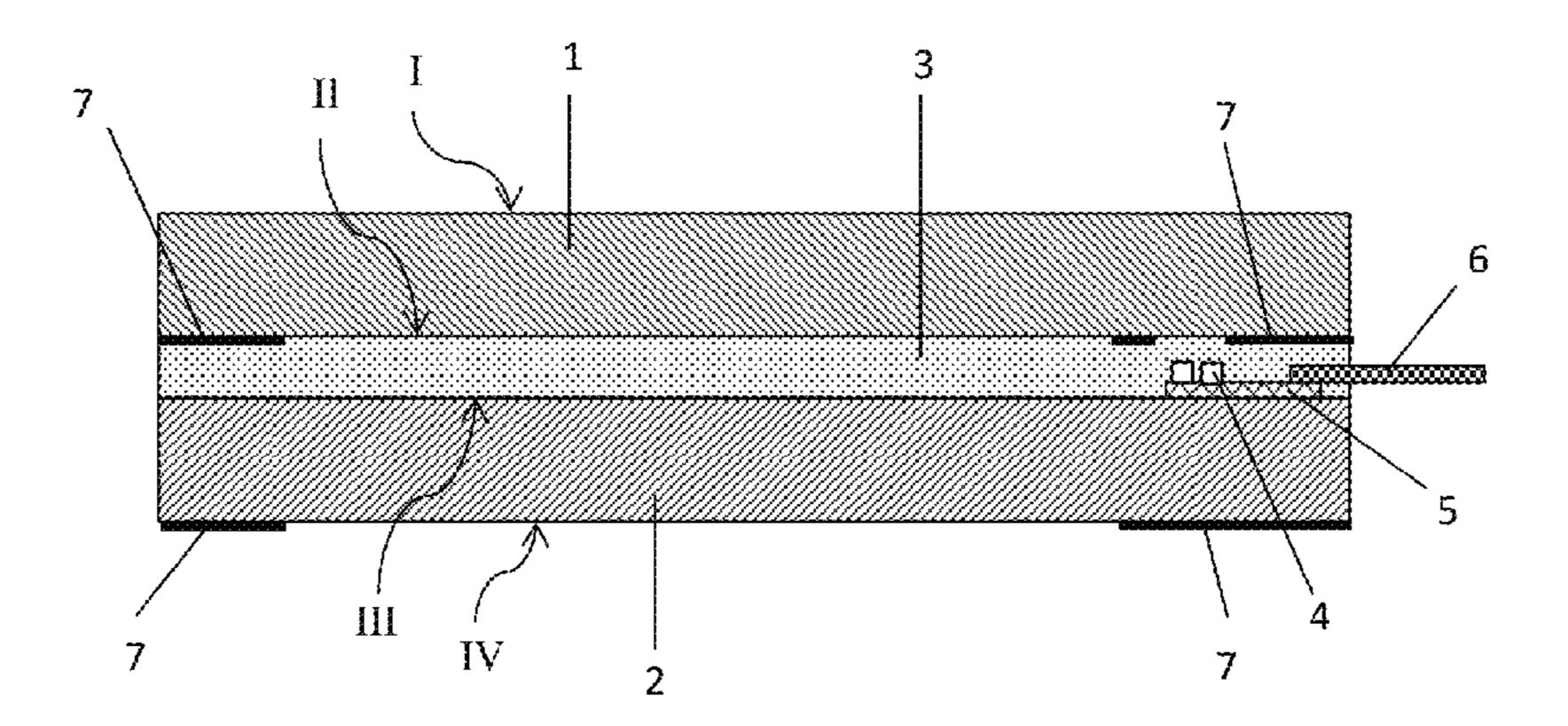
mounted device (SMD) components. The photodiodes are arranged on the circuit board as groups of parallel connected photodiodes. All groups of the parallel connected photodiodes are connected to a common electrical input and each group is connected to a separate electrical output.
