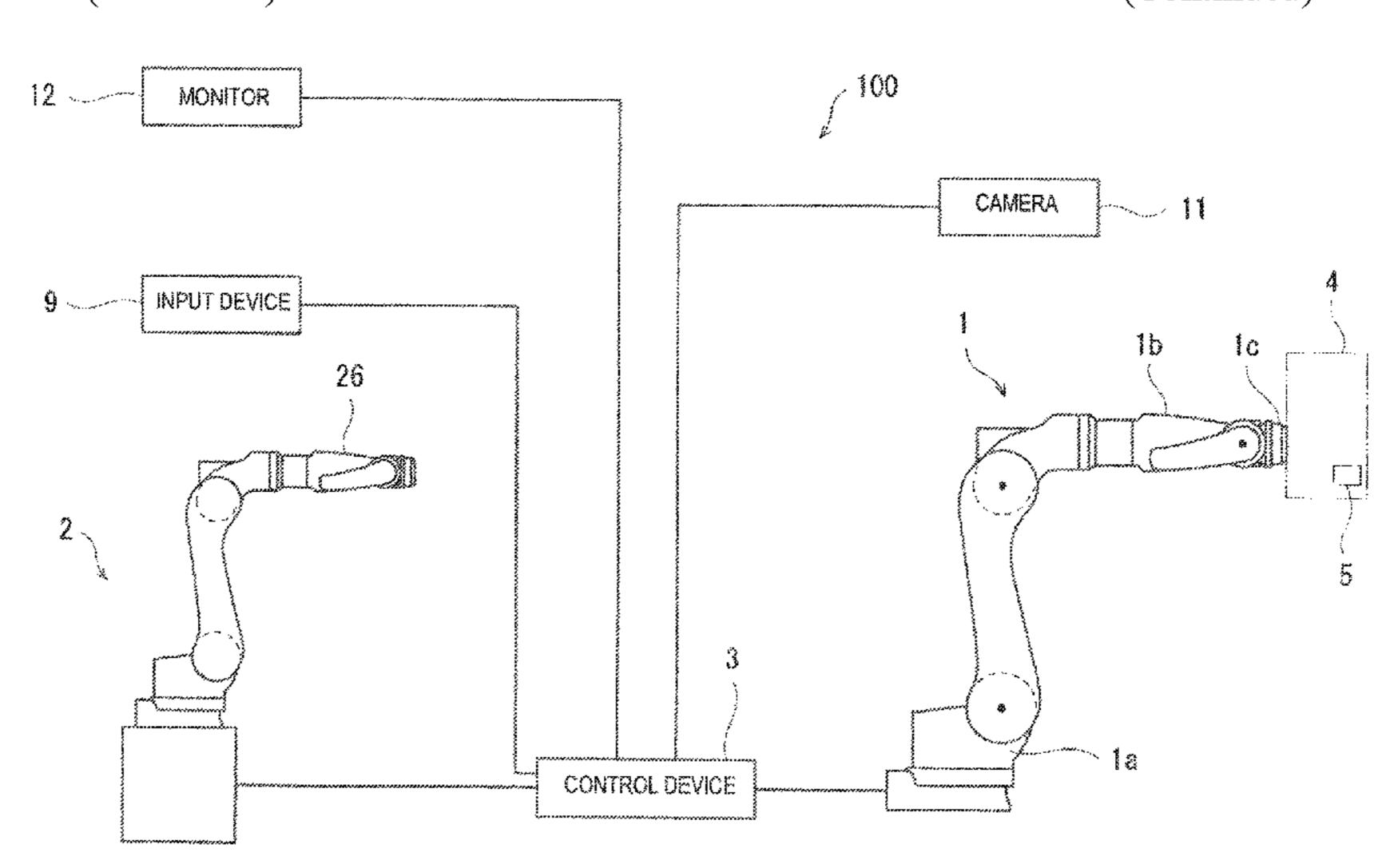
correlation to the velocity at the tip end of the end effector, as virtual reaction-force information, and a force applying device configured to give a force to the operating part in order to make an operator perceive a force according to the virtual reaction-force information outputted from the virtual reaction-force information generating module.
