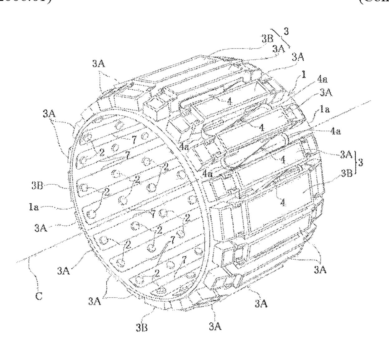
electric detection electrodes; and connection cables that electrically connect mutually adjacent myoelectric detection units and thereby transmit the myoelectric signals. The connection cables each include a bent portion, the bent shape of which changes in response to changes in the distance between the mutually adjacent myoelectric detection units.
