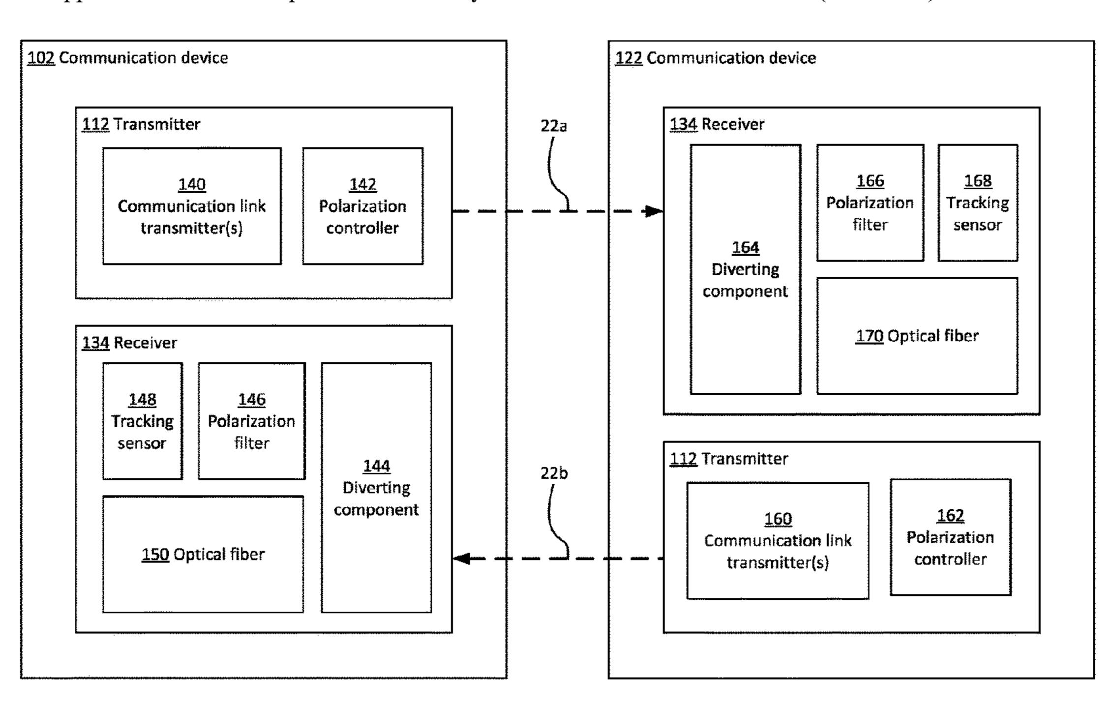
device to a second communication device. At the second communication device, the polarized optical communication beam is processed to extract the encoded information, and the encoded information is used at the second communication device to track the optical communication beam.
