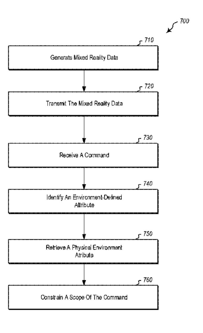
architectural element. Additionally, the computer system constrains a scope of the command based upon an interaction between the virtual architectural element and the real-world environment.
