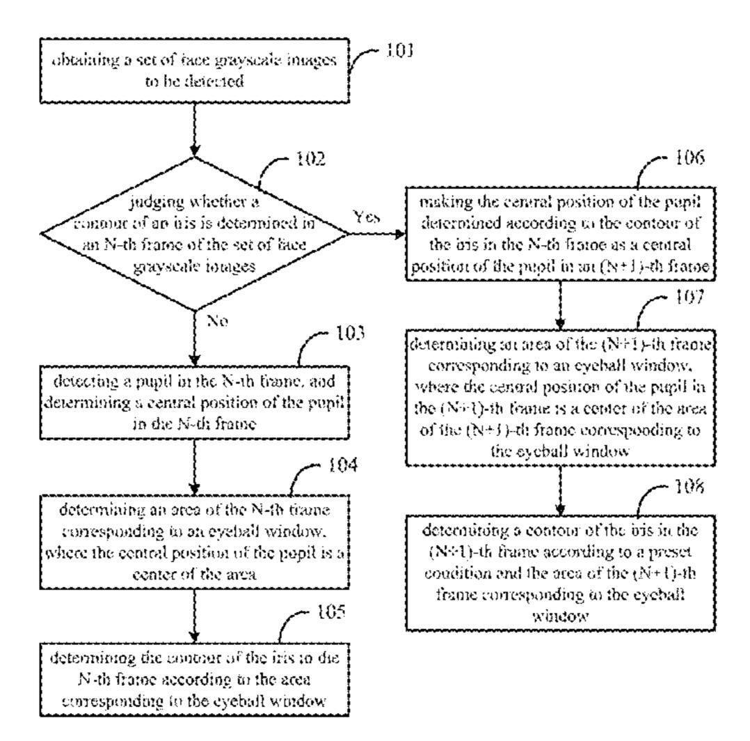
eyeball iris in the N-th frame facial grey-scale image (105). By judging that the contour of an eyeball iris is not determined in a facial grey-scale image, the tracking of the contour of the eyeball iris can be automatically adjusted, and an eyeball pupil is positioned again. By means of the present invention, the accuracy rate of eyeball tracking is improved, and an eyeball can be automatically identified to detect the central position of an eyeball pupil.
