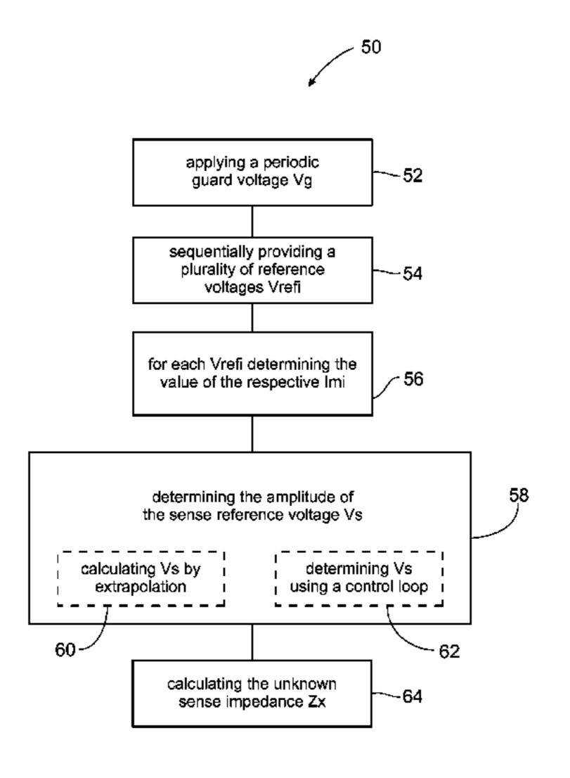
electrode, with reference to the sense reference voltage Vs, the periodic guard voltage Vg, and the reference impedance Zref.
