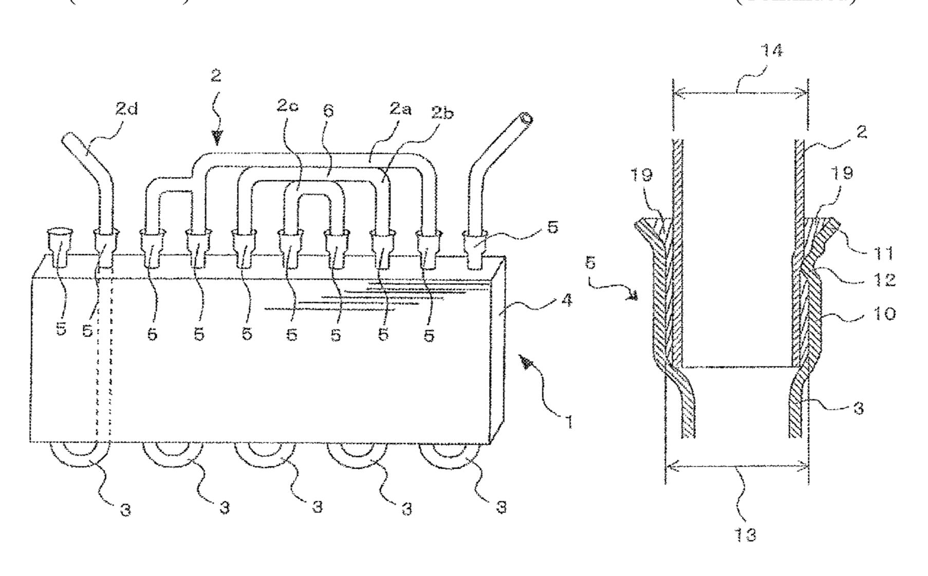
flare, and the pipe component has a groove formed by the at least one protrusion.
