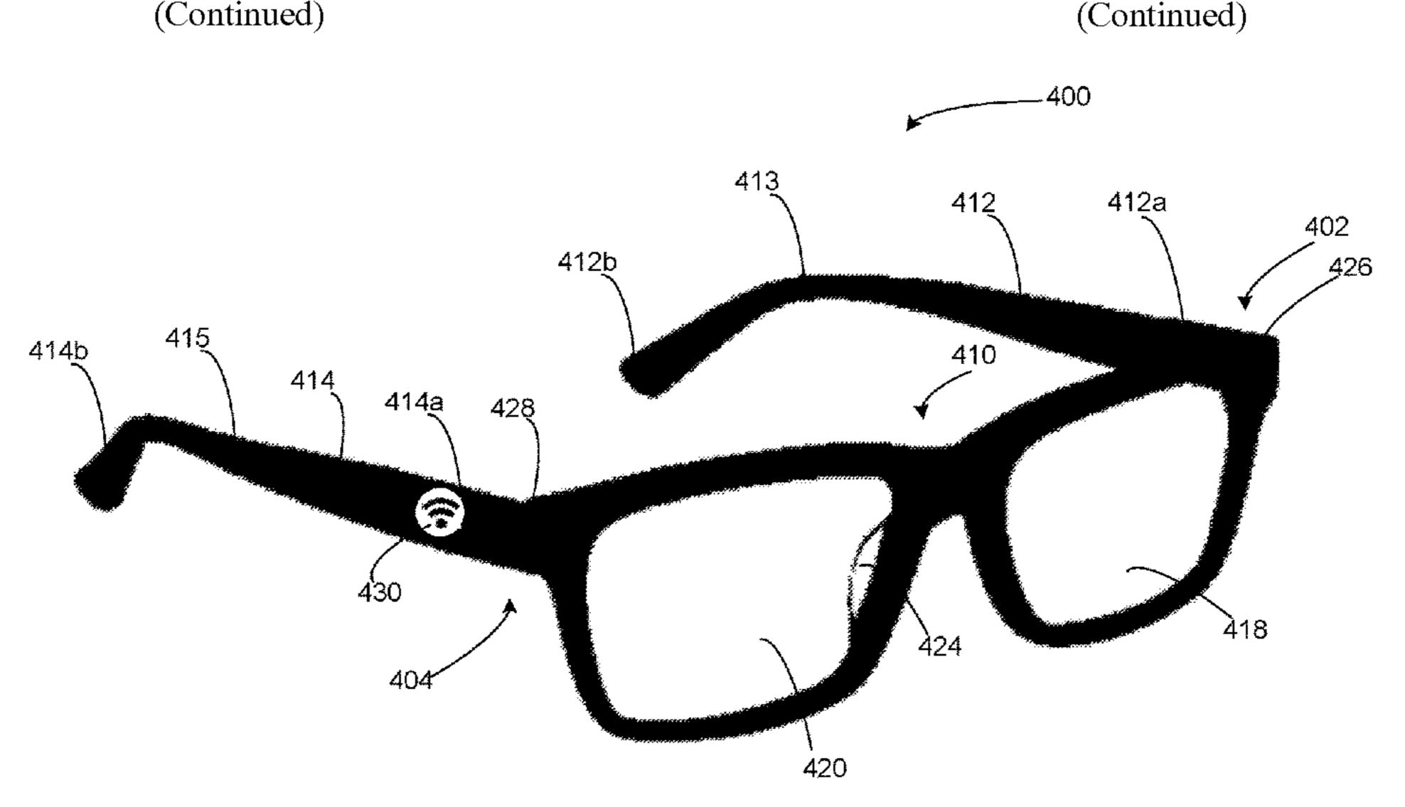
computerized wearable device may detect one or more of the wearer's physiological characteristics (e.g., oxygen levels, pulse rate, pupil size, etc.) and determine the wearer's alertness level.
