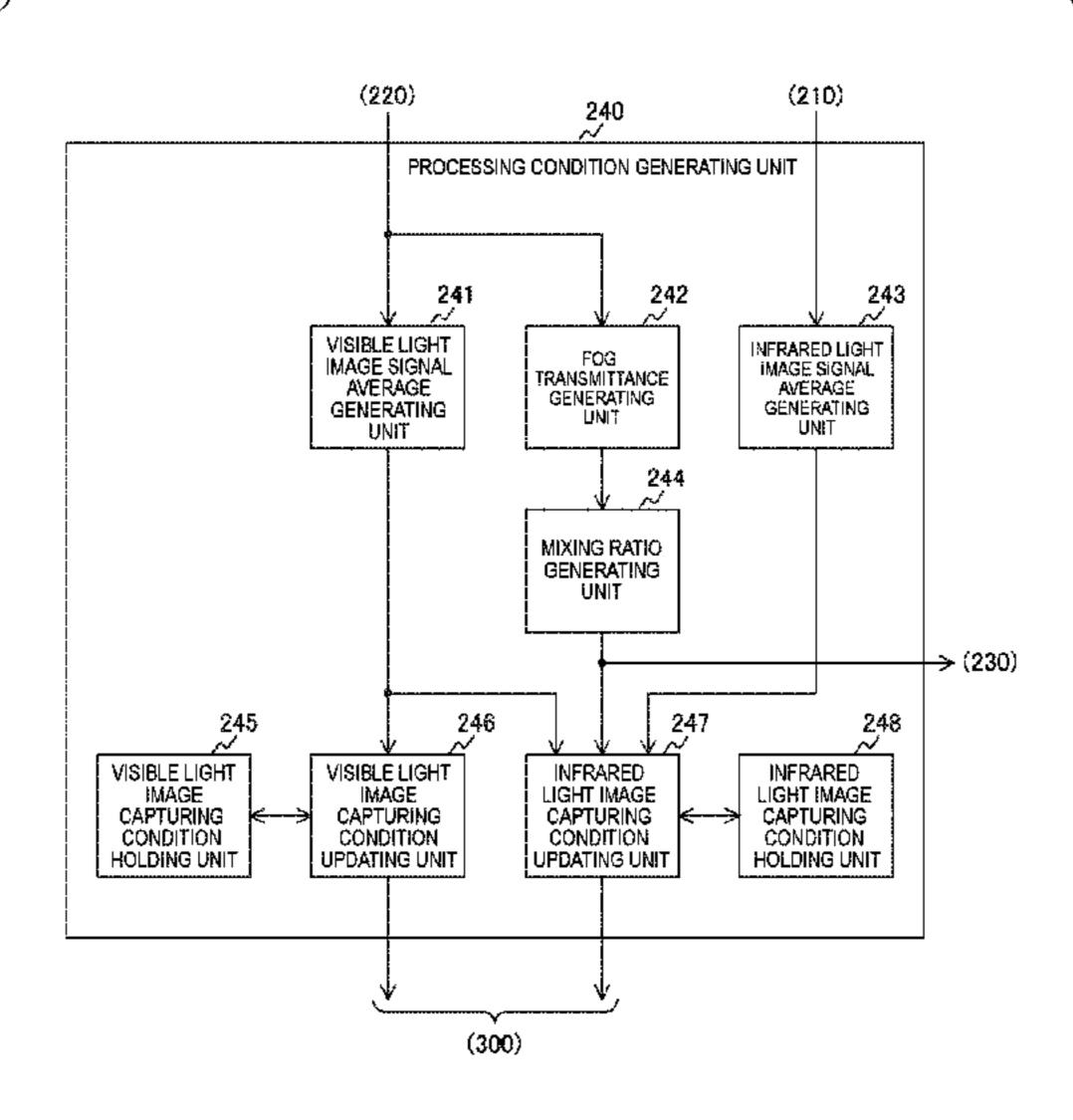
is mixed with a non-visible light image signal in the region, and image capturing conditions of the non-visible light image signal in the region are updated.
