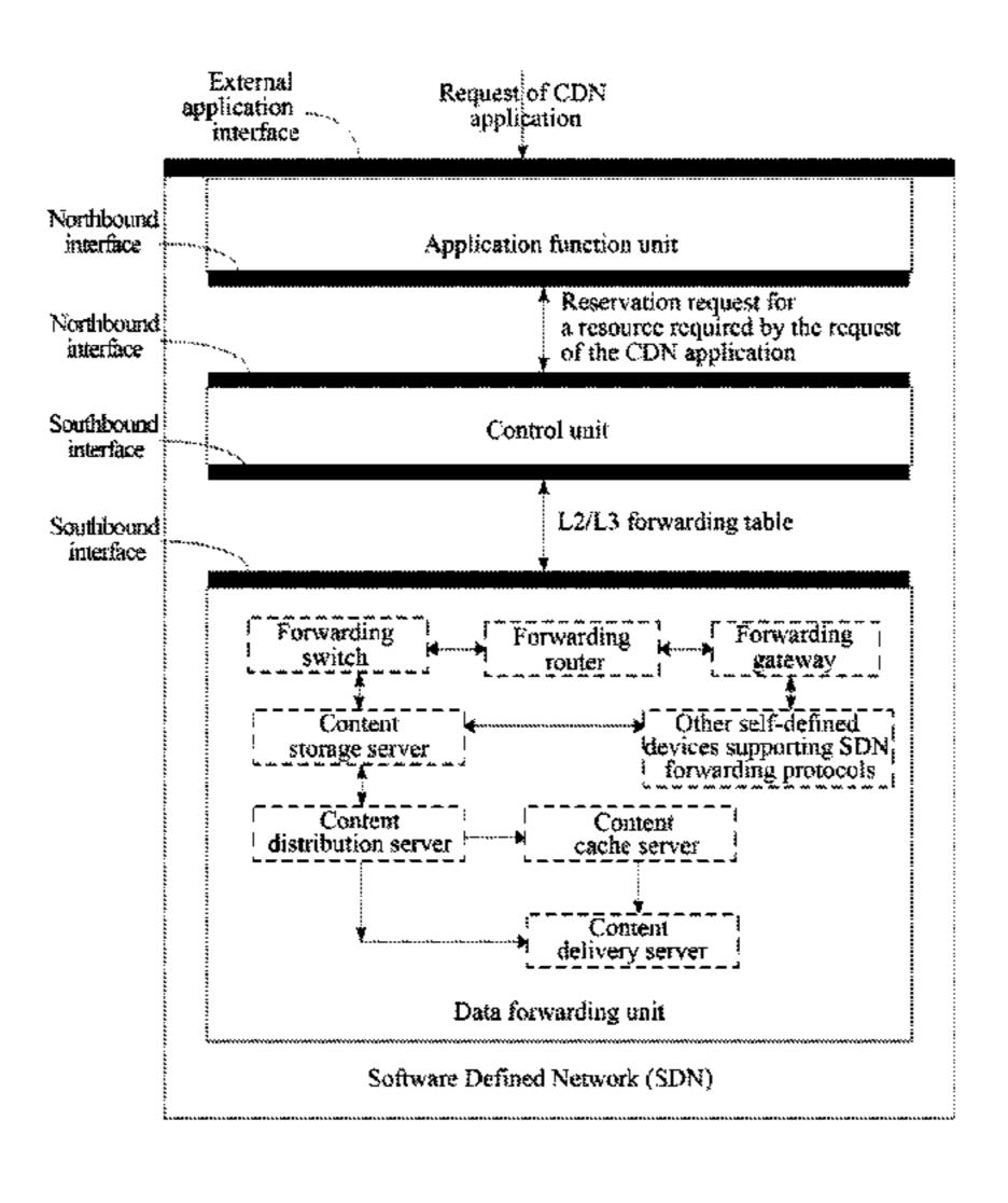
work load balancing and path policies and to generate a content routing table for data transmission, generating and transmitting L2 and L3 forwarding tables to the SDN data forwarding layer. When it receives content distribution and content delivery requests, the SDN data forwarding layer executes a CDN service-related operation based on the forwarding tables.
