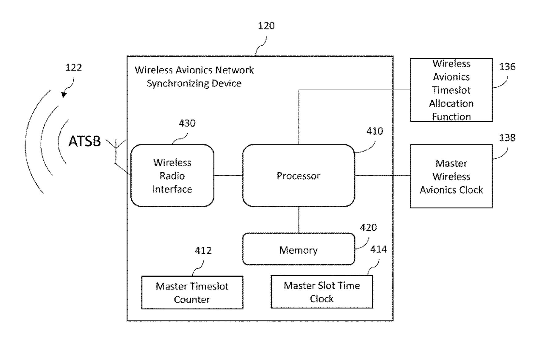
wherein the network synchronizing device broadcasts an arbitrary timeslot synchronization beacon to the plurality of device nodes on the first designated synchronization channel in the timeslot; wherein the arbitrary timeslot synchronization beacon comprises a Sync Timeslot identifier that identifies the timeslot, and a Sync Time indicator that includes a time that the arbitrary timeslot synchronization beacon was transmitted.
