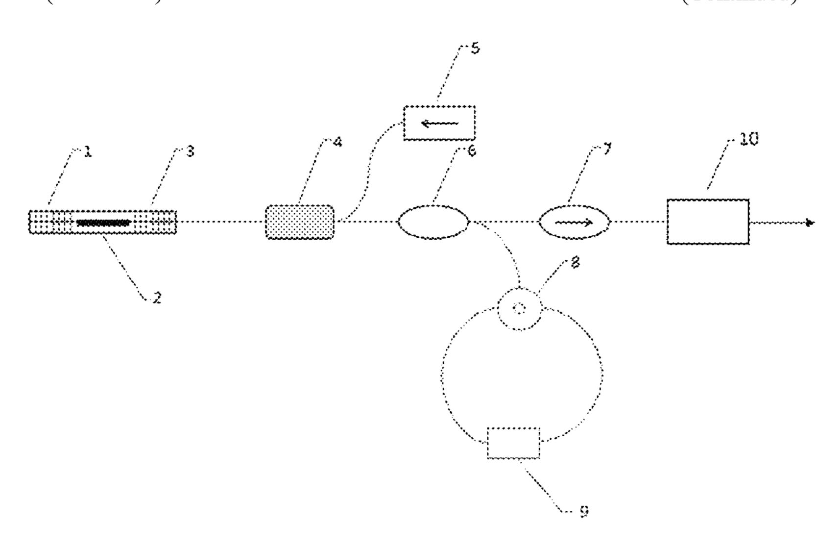
optical fiber. A portion of the wide-spectrum laser is filtered by the optical filter module to obtain a wavelength corresponding to a specific central frequency. Multi-wavelength laser lasing with a narrow linewidth and single longitudinal mode is implemented by combining a short linear resonant cavity structure and the optical filter module.
