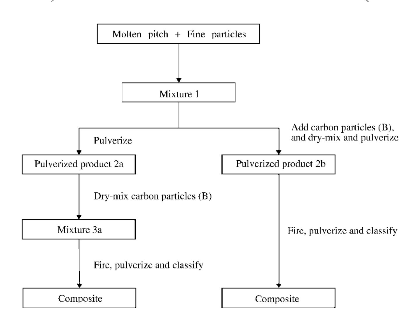
followed by dry mixing and pulverizing, to obtain a pulverized product (2b); and firing the pulverized product (2b), followed by pulverization.
