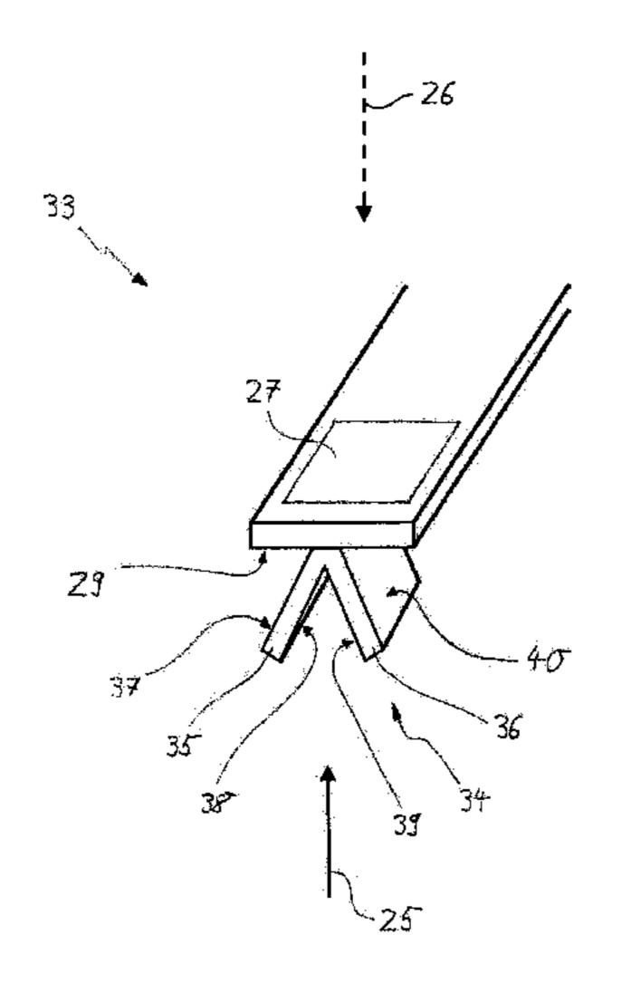
has a reflection surface (27) on a side facing away from the inflow structure and the measurement apparatus (16) has a laser (17). A beam axis (26) of the laser (17) is directed to the reflection surface (27) of the boom.
