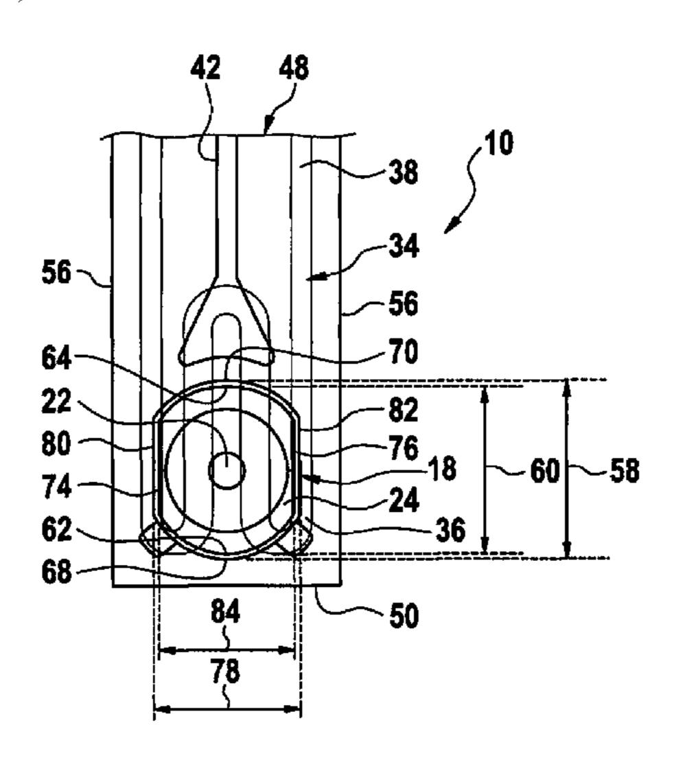
construction. The second electrode has at least one outer diameter that is greater than a corresponding outer diameter of the electrode cavity.
