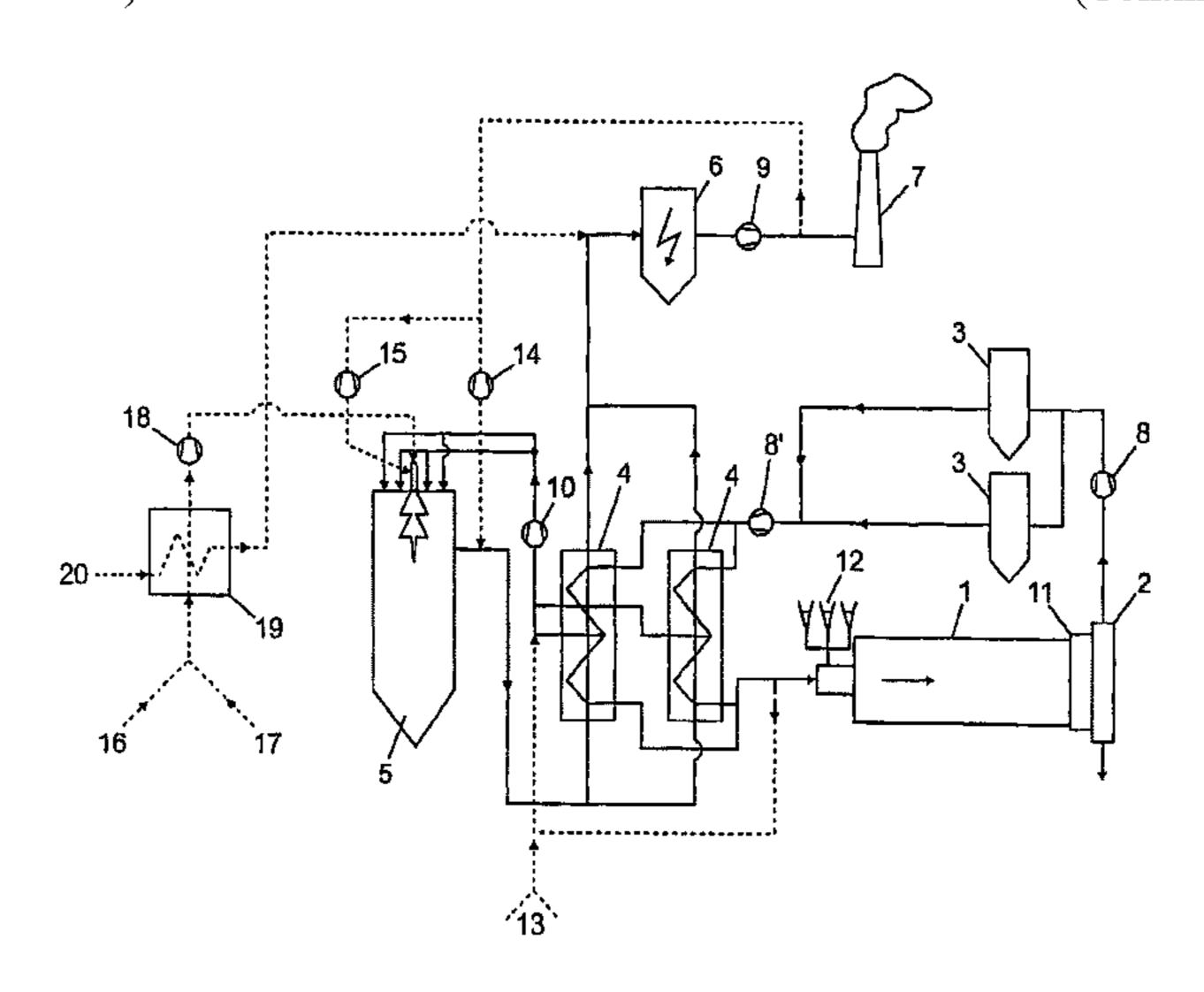
least one heat exchanger (4), at least a partial flow of the drying vapors are branched off to be conducted into the burner (5). The remaining partial flow is conducted to the dryer (1) again. The partial flow of drying vapors to the burner (5) is driven by at least one regulable partial vapor fan (10).
