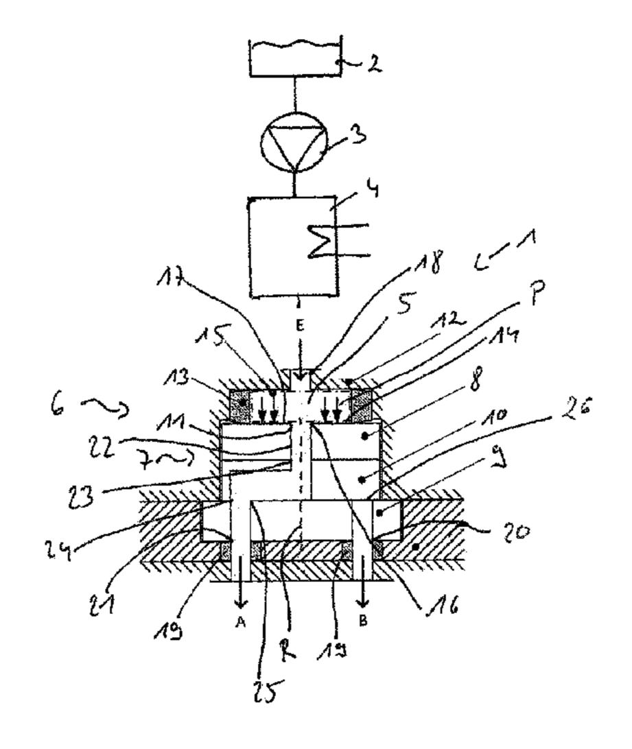
(13) and/or the pressure-surface portion (17), able to be loaded with hydraulic pressure, of the outer cover disk (8) next to the fluid opening (11) corresponds to at least 20% of the axial projection surface of the cover disk (8), and/or is greater than a fluid-opening cross-sectional area of the fluid opening (11).
