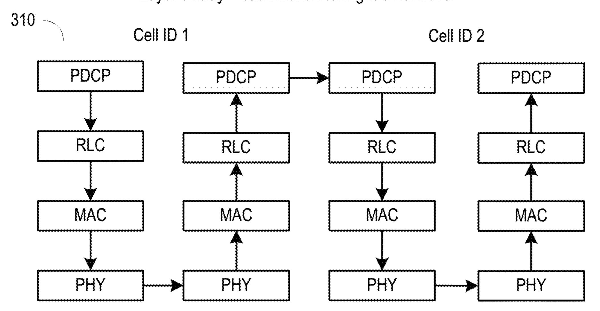
Layer 2 relay (switching enabled in the MAC/PHY layer)
