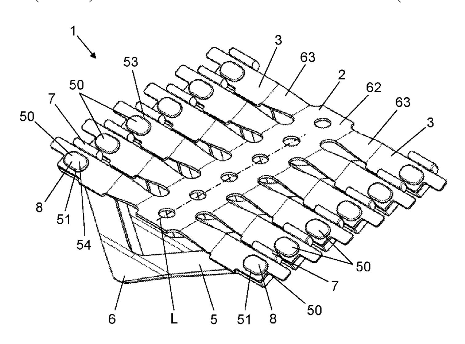
to the support strip (2) at a fastening point (3). Each contact part (5, 5a, 5b) comprises at least one plastically deformable connection element (50) for securing the contact part (5, 5a, 5b) to the support strip (2). The at least one connection element (50) forms an integral part of the contact part (5, 5a, 5b).
