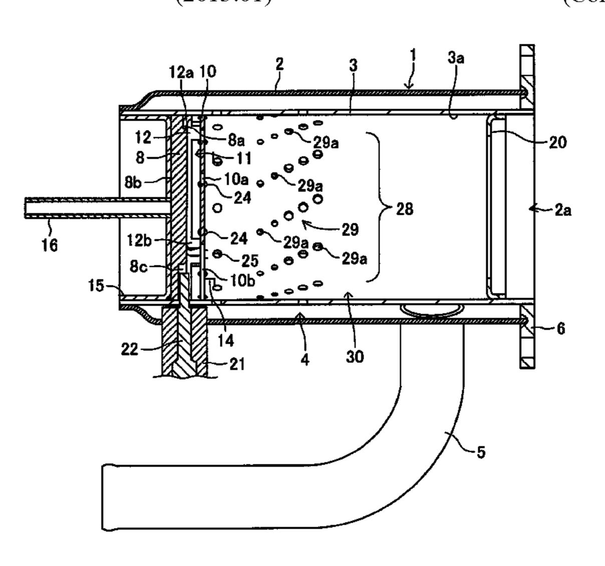
second air supply opening becomes larger toward the downstream side. Thereby, ignitability in an evaporation type burner is improved and incomplete combustion of fuel on the downstream side of the combustion chamber is reduced.
