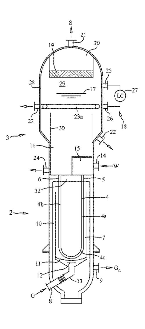
rated medium at least partially by gravity; the apparatus also comprises means for controlling the liquid level in the collection chamber and for a partial recycle of the nonevaporated liquid.
