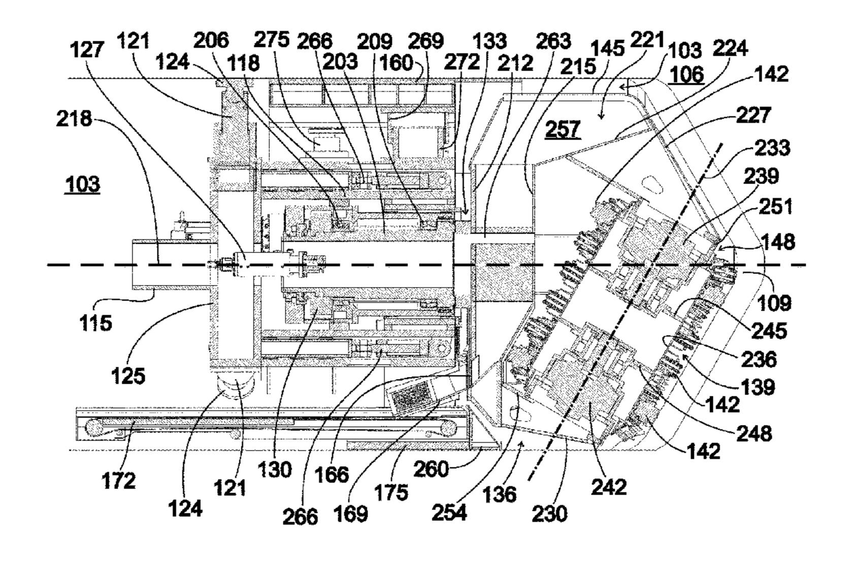
tion drum, the connecting arrangement being configured in such a way that the drum rotational axis and the longitudinal axis lie in a plane, and are oriented at an acute angle with respect to one another in the advancing direction, in all operating positions during the advancement, characterized in that the extraction drum extends over at least an effective radius of the device in the radial direction of the device during advancement of the cavity.
