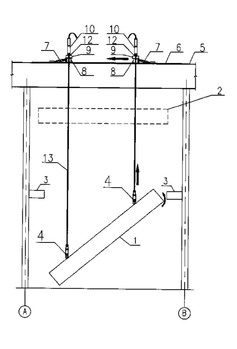
posture of the structure can be altered by operating the push instrument kits and the lifters, such that the horizontal projection of the structure will be reduced and the structure can therefore be lifted over the obstacle in vertical direction.
