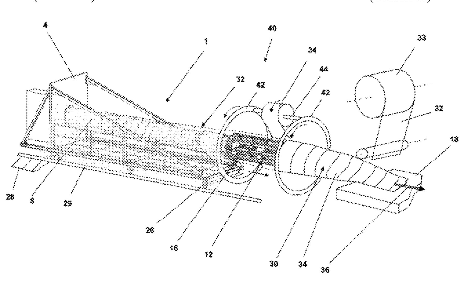
during the circumferential winding of the fiber strips (34), transports the inner film hose (32) in a feed direction (36) to a stationary supporting surface (18) which is arranged at the free end (10) of the winding mandrel (12) and over which the liner hose (30) is conveyed further, wherein the inner film hose (32) is drawn over the free end (13) of the winding mandrel (12) onto the support tube (8) against the feed direction (36).
