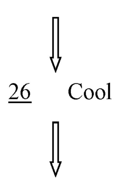
Cold Roll to Final Thickness (20-35% Reduction)
