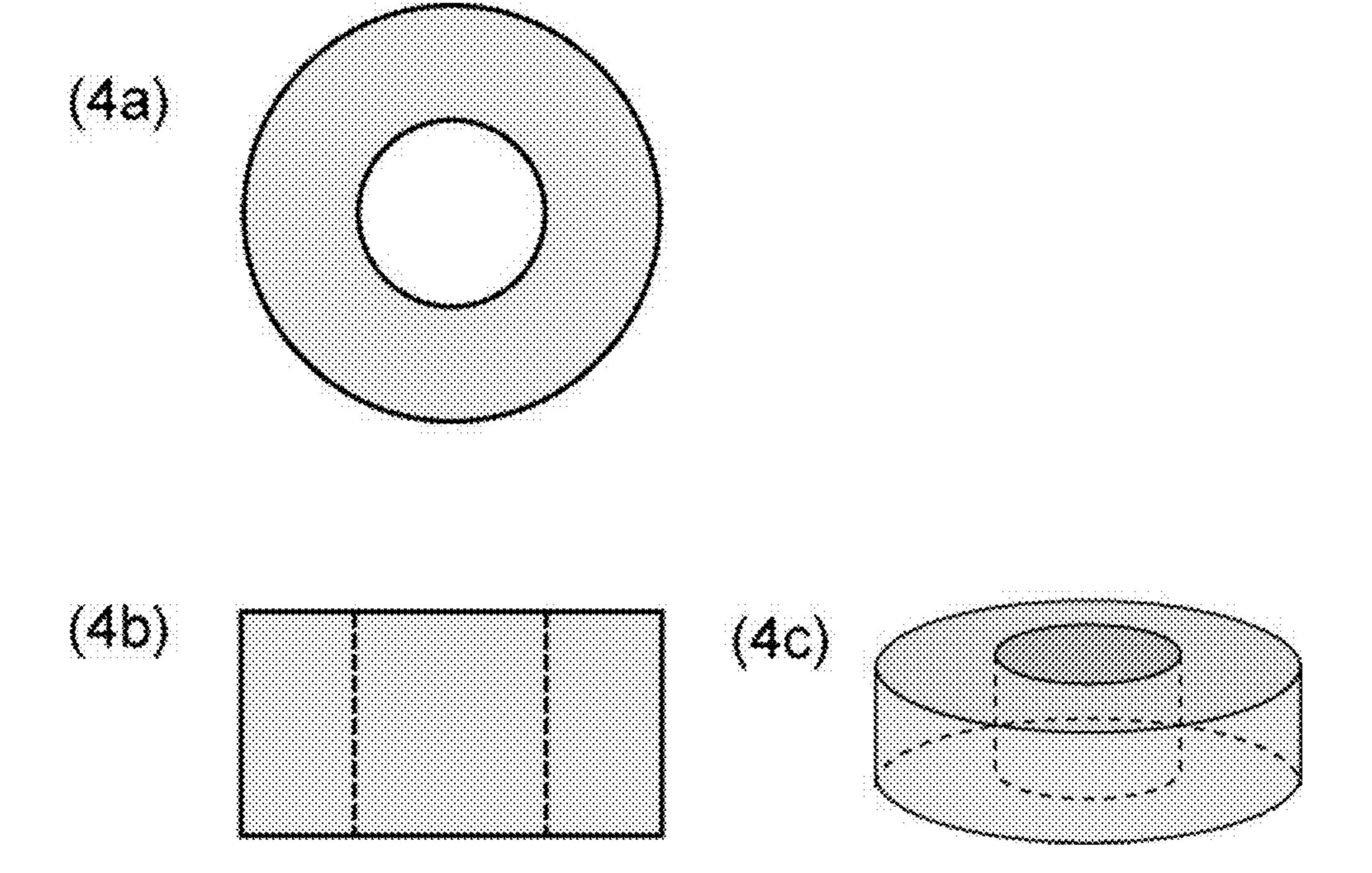
Figure 4 a-c. Sacrificial part of the sacrificial anode according to the invention.
