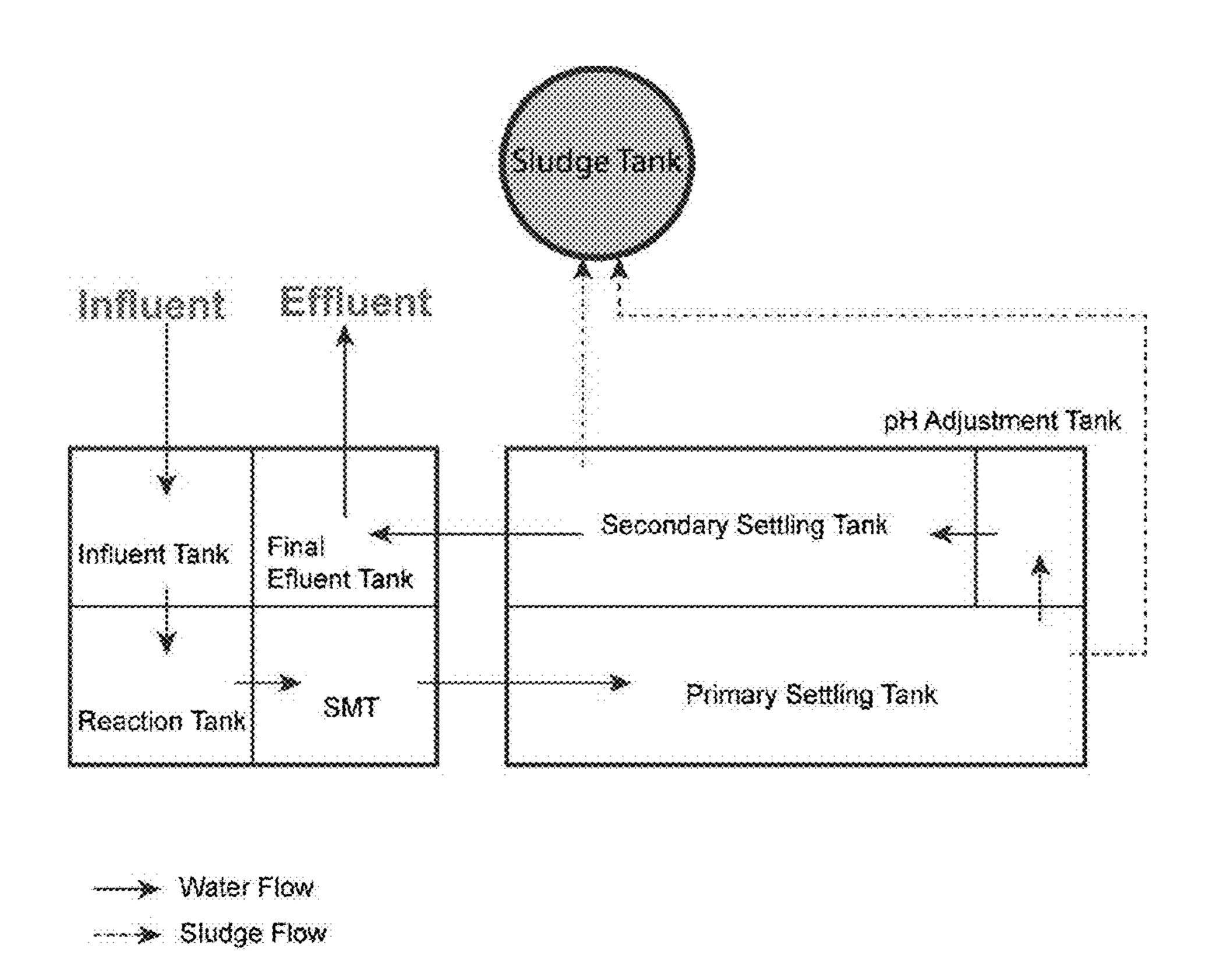
Figure 7. Principle flow chart of the electrocoagulation process according to the invention.
