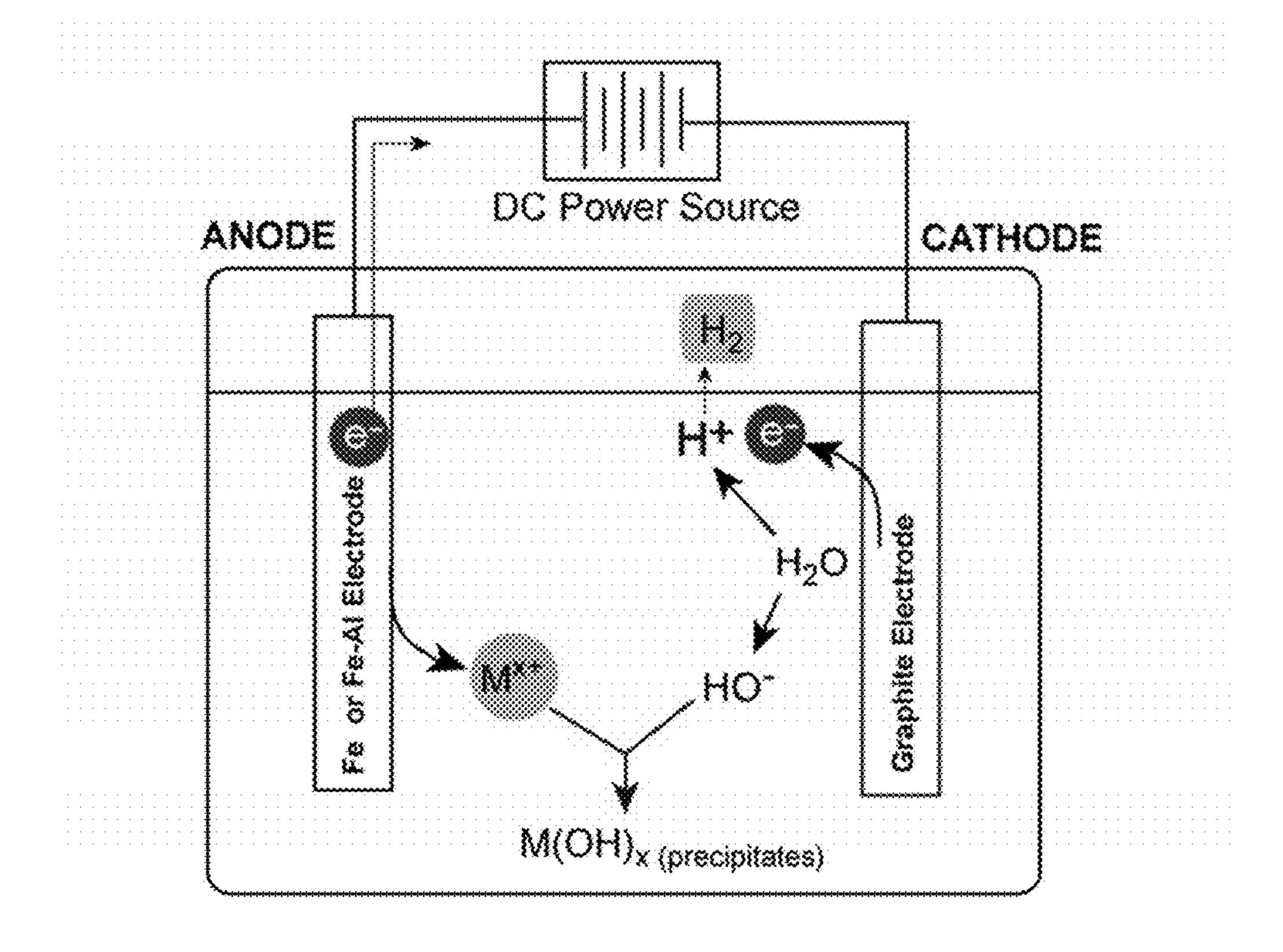
Figure 1. Principal drawing of the electrocoagulation process
