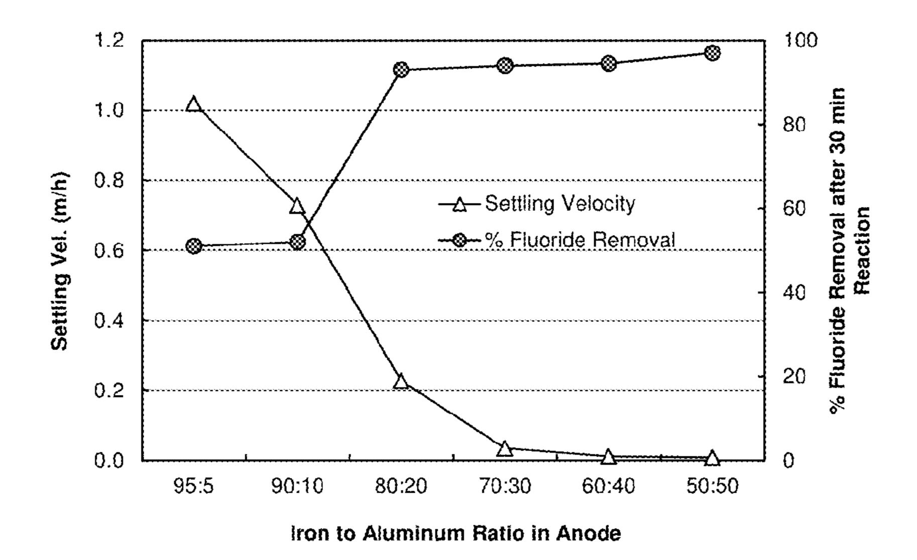
Figure 5. Settling velocity and fluoride removal capacity as a function of Iron to Aluminum ratio.
