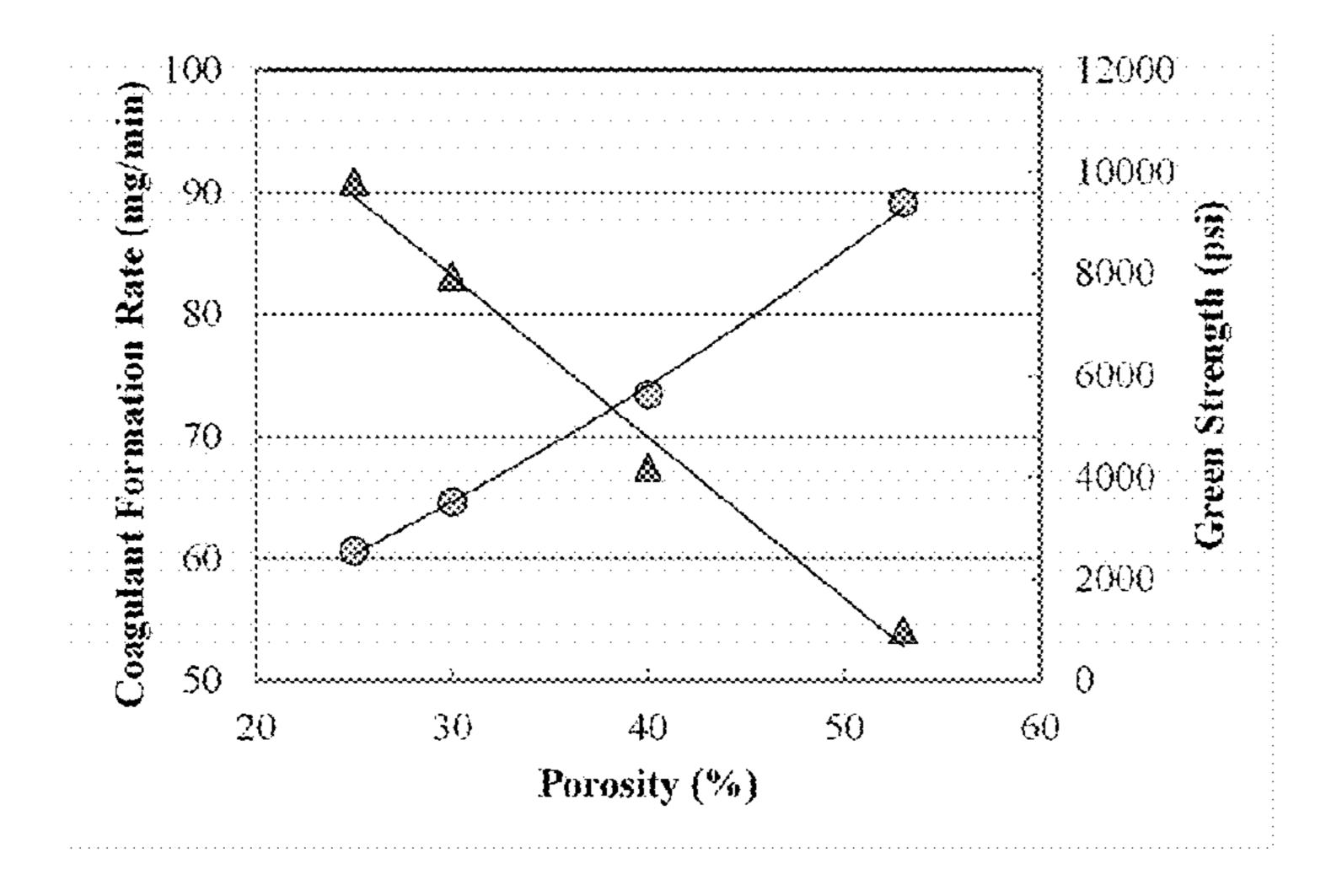
Figure 6. Rate of coagulant formation and Green Strength as a function of the porosity as described in example 5.
