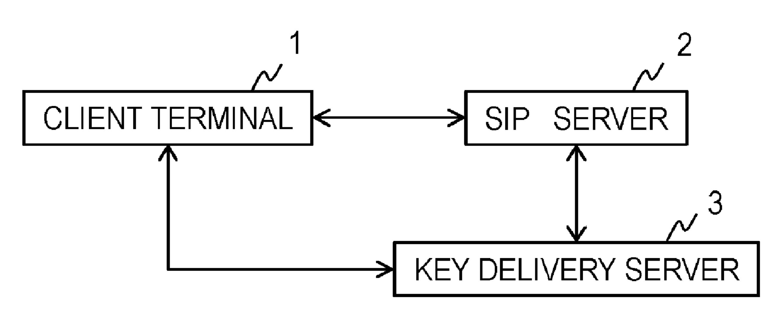
client terminal starts data transmission and reception by using the delivered key with a different client terminal from the aforementioned client terminal. The client terminal performs data transmission and reception with the different client terminal by using the delivered key.
