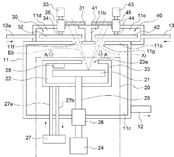
irradiating the target starting material with the energy beam, and allow the X-rays to proceed to the exterior of the chamber.
