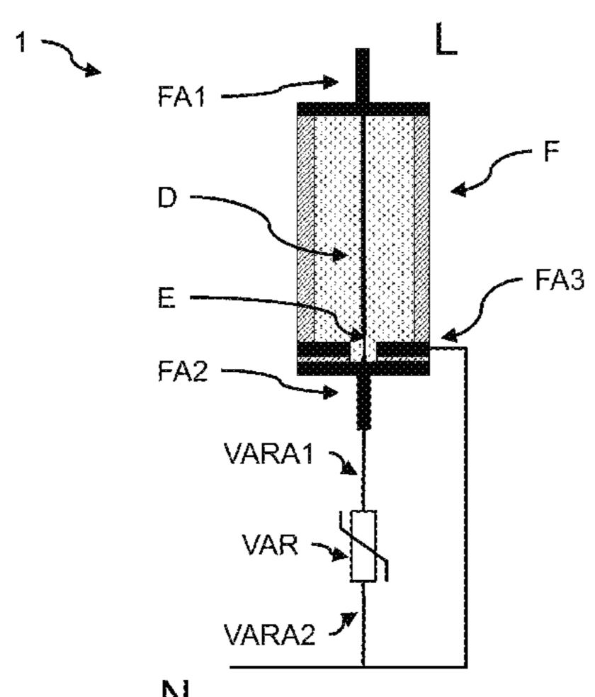
ing to a load below the type-II rating do not result in a lasting change in the constriction, wherein the constriction, in conjunction with the fluxing agent, is dimensioned such that pulses corresponding to the limit range of the type-II rating result in the fusing of the fluxing agent into the fuse element, and wherein pulses corresponding to a load that is stronger and/or of greater duration than the type-II rating of the varistor result in the immediate disconnection of the fuse element.
