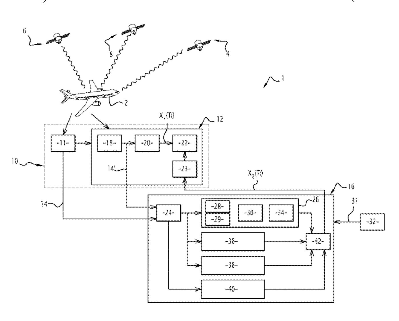
device being able to carry out processing of the received radio navigation signals to calculate first navigation information including information on the geographical position, speed and time of the carrier.
