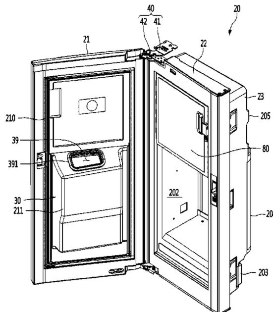
disposed on a front surface of the second door; and a discharge duct provided in the second door, wherein, when the second door is closed, the guide duct communicates with the discharge duct, and ice made in the ice making room is discharged to the dispenser.
