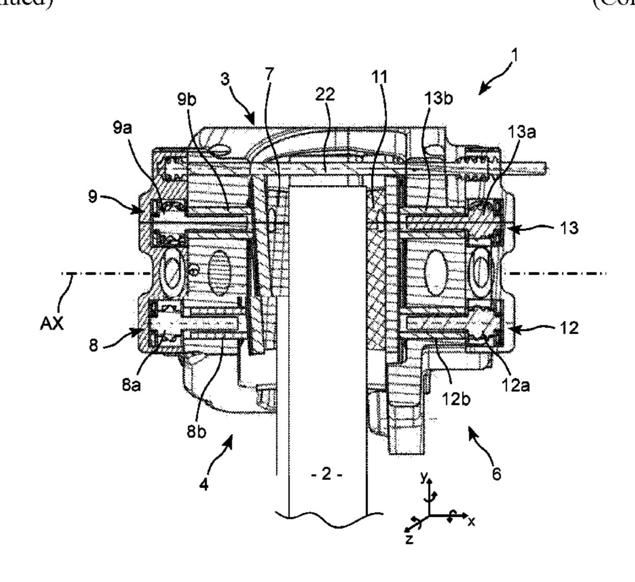
the two pinions with the two endless screws thereof each engaged in a pinion.
