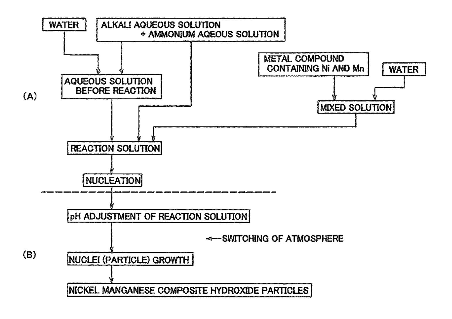
are grown by switching the atmosphere from the oxidizing atmosphere to a mixed atmosphere of oxygen and inert gas in which the oxygen concentration is 1% by volume or less.
