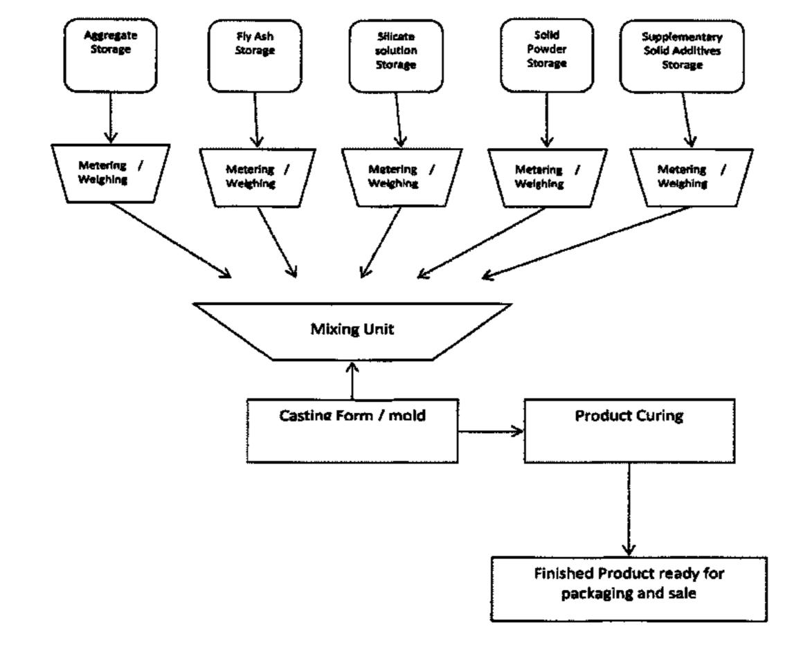
condensation reaction proceeds and the activated geopolymer premix stiffens to produce a self-supporting cellular structure; and (d) curing the self-supporting cellular structure to produce the cellular geopolymer product, wherein in step (c) the characteristics of the activated geopolymer premix and the reaction kinetics of the condensation reaction are controlled to achieve formation of the self-supporting cellular structure.
