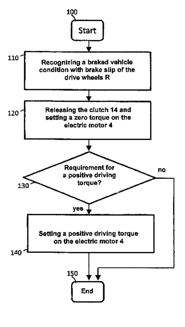
torque on the electric motor is produced by the torque of the internal combustion engine and the torque of the electric motor. The presence of a specific vehicle condition indicative of brake slip of the drive wheels or a risk thereof is recognized. If such a vehicle condition is recognized, the clutch between the internal combustion engine and the electric motor is released and the torque of the electric motor is increased.
