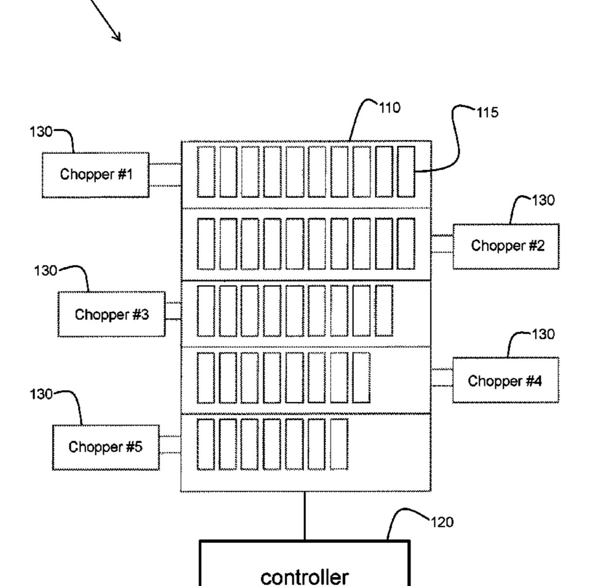
configured to support reconfigurable parallel electrical connections of subsets of the power supply modules. Each subset is configured to electrically connect to an output power supply stage to provide a dynamic waveform-controlled welding or cutting electrical signal to support generation of a single arc between an electrode and a workpiece.
