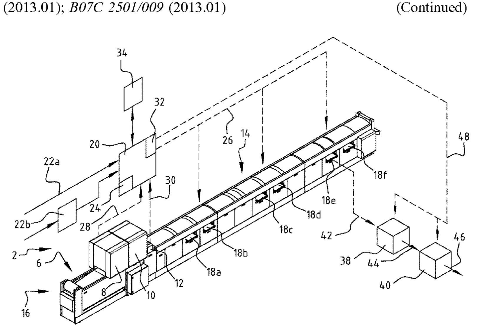
cation system is configured to distribute assessed products over the qualifying sorting outlets in the task configuration.
