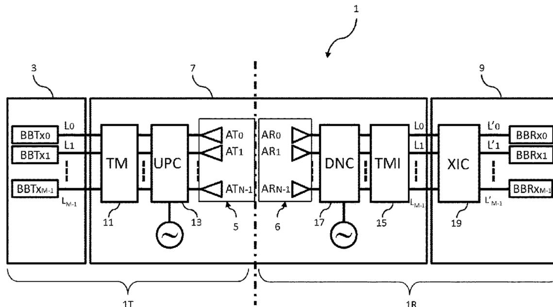
(OAM), wherein the device is adapted to receive, at its input, electromagnetic signals from at least one transmitter, and is configured to apply a discrete Fourier transform to the electromagnetic signals in order to generate the signals having electromagnetic modes with orbital angular momentum.
