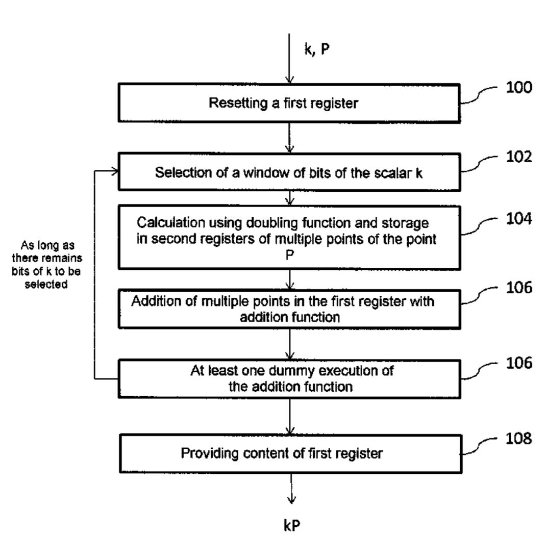
the bits of the window during an iteration of the loop are non-zero, the multiple points to be added in the first register during the step are determined from a non-adjacent form associated with the window.
