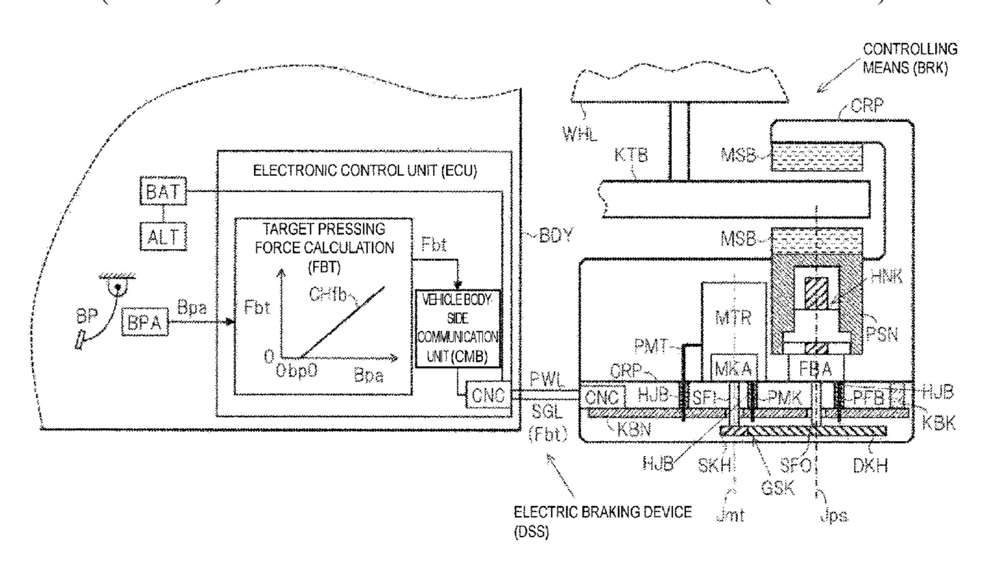
into the circuit board KBN, which is fixed to the caliper CRP by the holding member HJB and the motor pin PMT.
