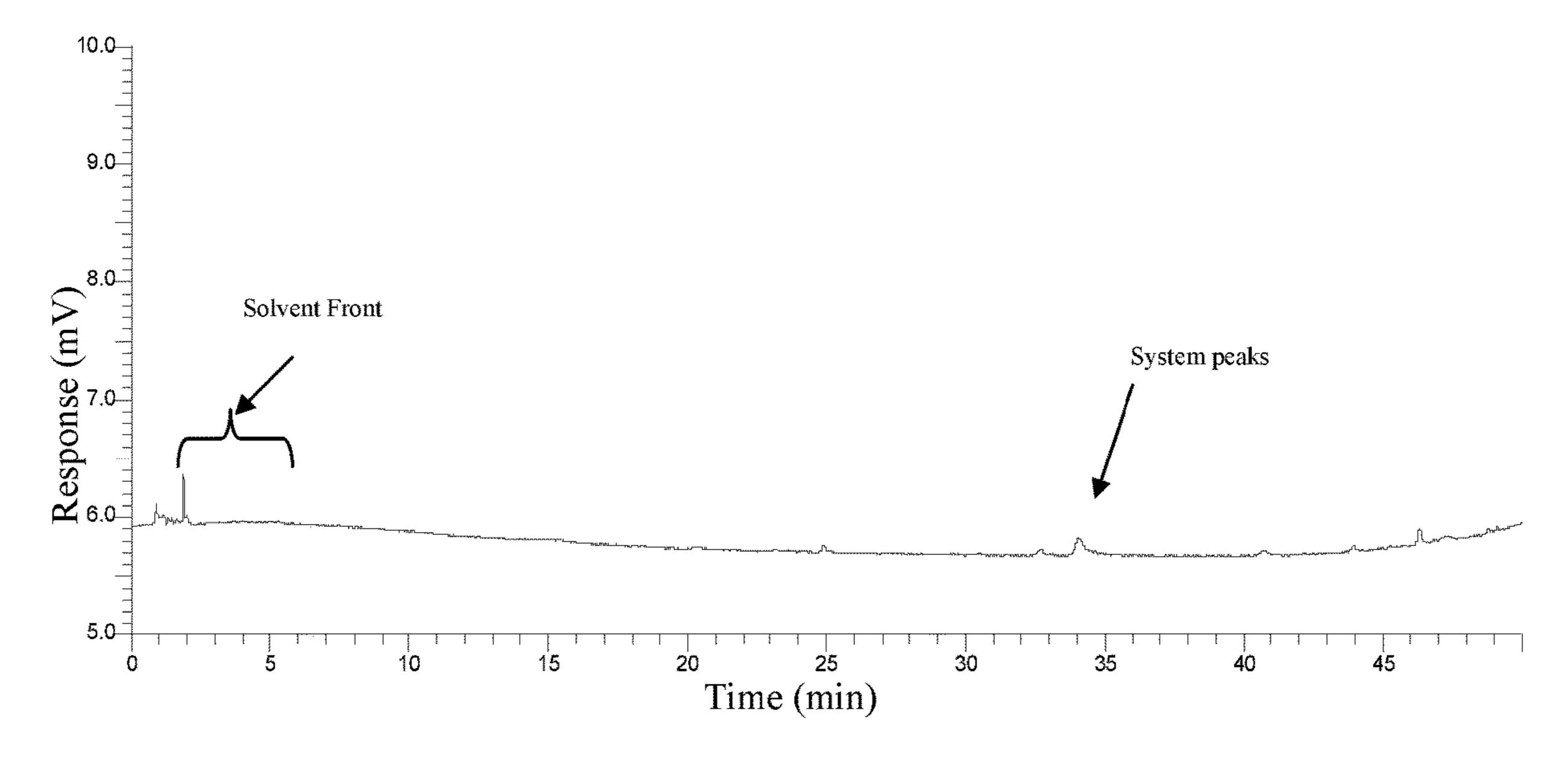
NOTE: Chromatogram solvent peak and system peak can be instrument dependent.
