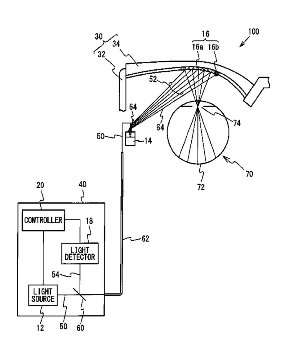
from a direction in which the image light beam is reflected, and scanning neither the image light beam nor the detection light beam reflected by the first mirror; a detector detecting the detection light beam reflected by the second region; and a controller adjusting oscillation of the first mirror and an emission timing of the image light beam based on a detection result by the detector.
